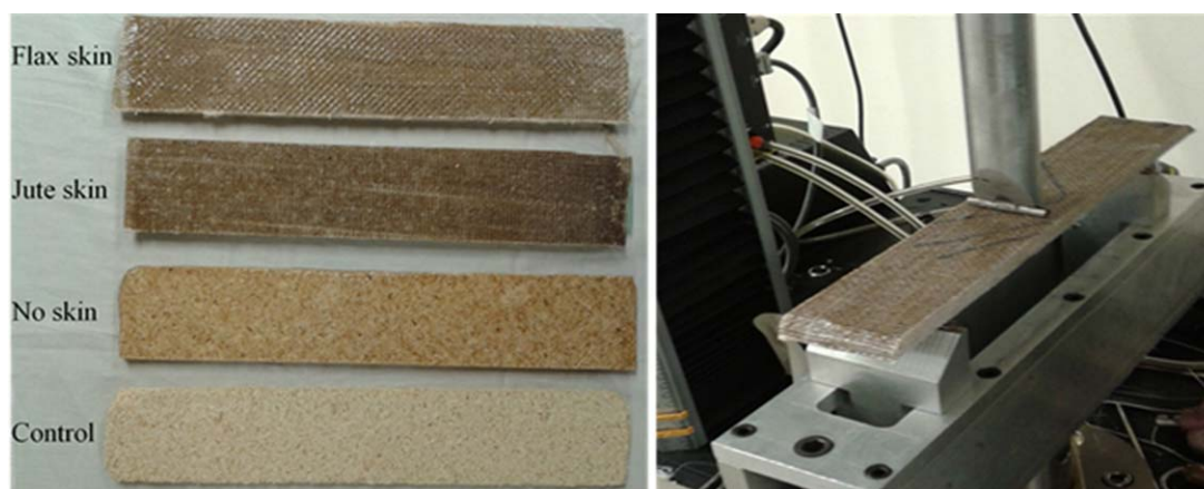
Figure 4. 3-point bending test: (a) test specimens and (b) 3-point bending test set up. [Color figure can be viewed in the online issue, which is available at wileyonlinelibrary.com .]
